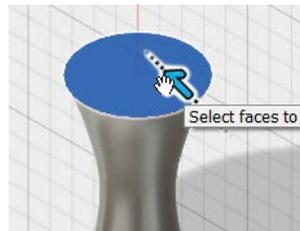
3. Rotate the model to view the bottom face, and then select the bottom face.
