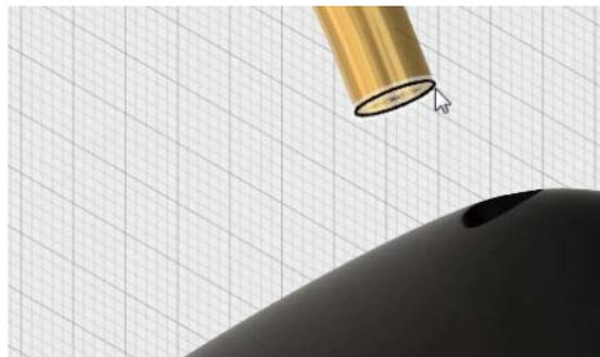
15. Rotate the model to view the edge of the hole in the stand. Select the center of the circle as shown.
