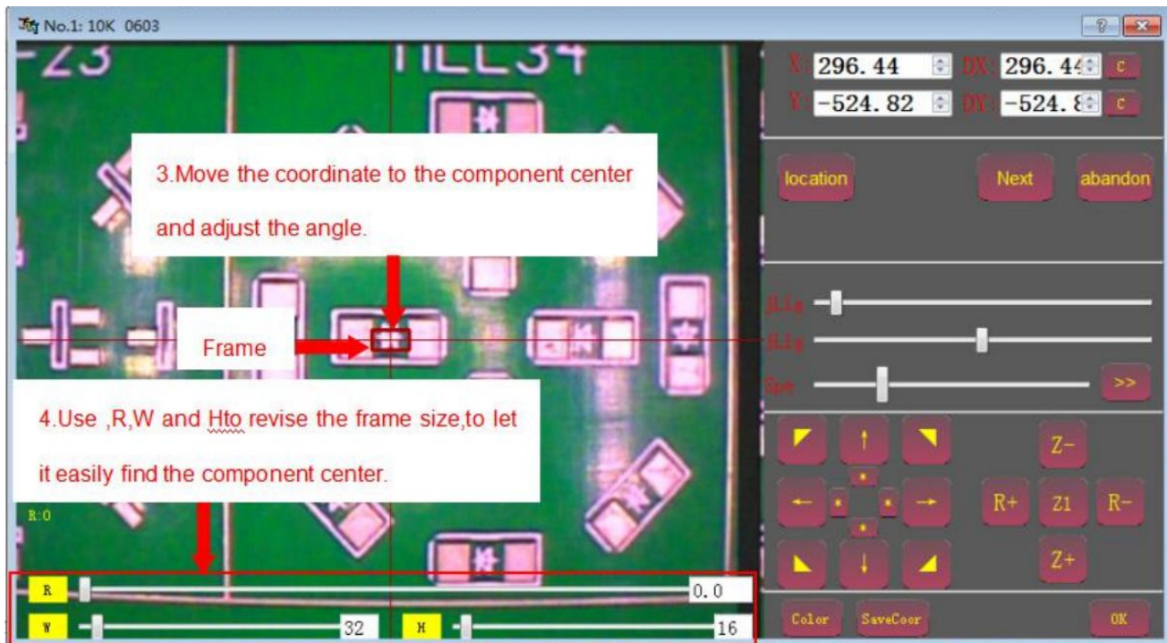
Fig.3-21 Manual edit SMD component
